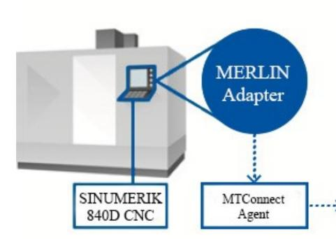
This schematic illustrates the typical scenario for a machine tool control modification at an end-user, where the Memex Automation software is added to the SINUMERIK CNC, allowing machine data to be sent through an agent in MTConnect-compatible language. This facilitates a significantly greater degree of information gathering and analysis by the customer across the open-source standard of MTConnect for greater interoperability between devices and software applications.
